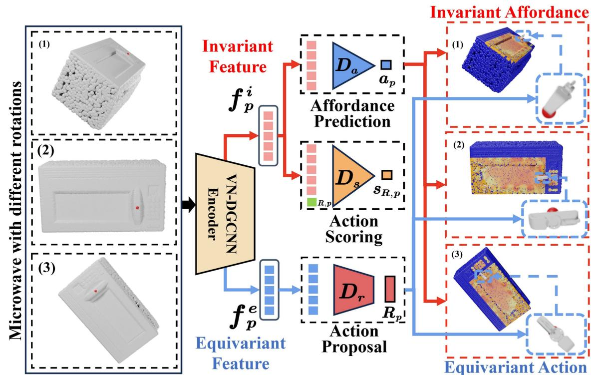
Taking as input a point cloud of the object, our framework first outputs a per-point SE(3) invariant feature  $f_p^i$  and SE(3) equivariant feature  $f_p^e$ . The invariant  $f_p^i$  results in the affordance map invariant to object rotations, while the equivariant feature  $f_p^e$  results in the manipulation actions equivariant to object rotations.
