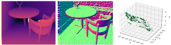
**Figure 1:** In surfel init stage, the input is the depth map. Initially, we calculate the gradient of the depth map using the Sobel operator to derive the normal map, as illustrated in the middle. Subsequently, the downsampled depth map is transformed into a point cloud utilizing the camera projection. The point position corresponds to the center of a disk, the normal determines the orientation of the disk, and the disk radius represents the uncertainty.
